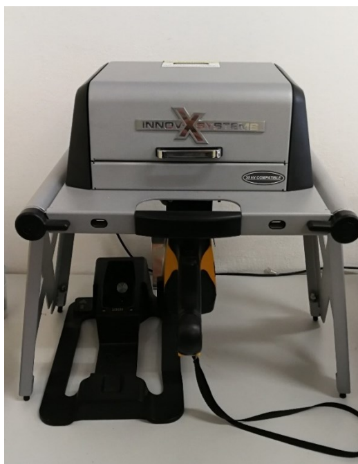
Slika 8. Olympus Portable X-Ray Fluorescence
