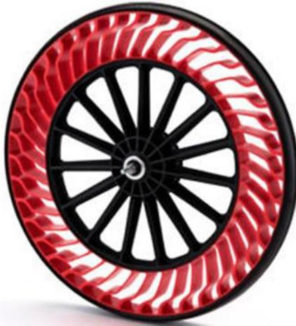
Slika 15 Bridgestoneov ne-pneumatski kotač
