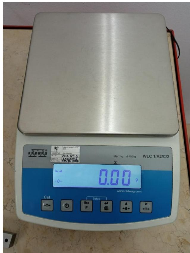
Slika 40. Digitalna vaga RADWAG WLC 1/A2/C/2
