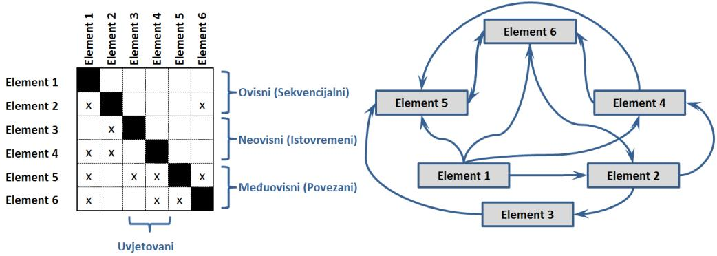
Slika 3.2. DSM (*design structure matrix*)
