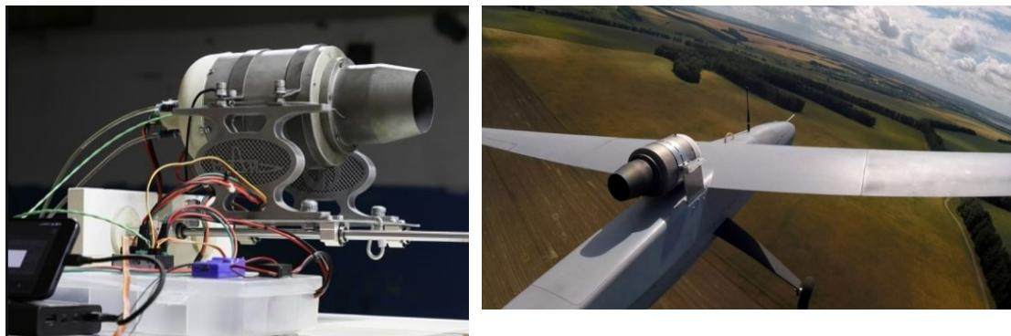
Slika 17. Plinsko-turbinski motor MGTD-20 [35]
