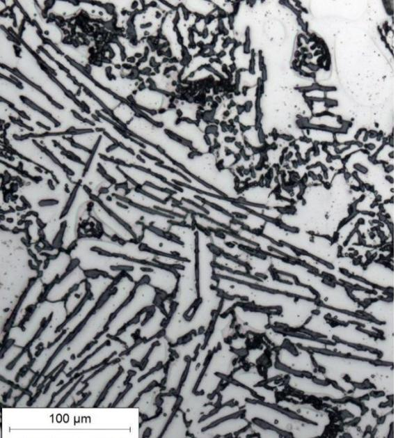
A micrograph showing a more irregular and fragmented distribution of dark, elongated precipitates compared to the polished surface. A scale bar in the bottom left corner indicates 100 μm.<br>100 μm             |
