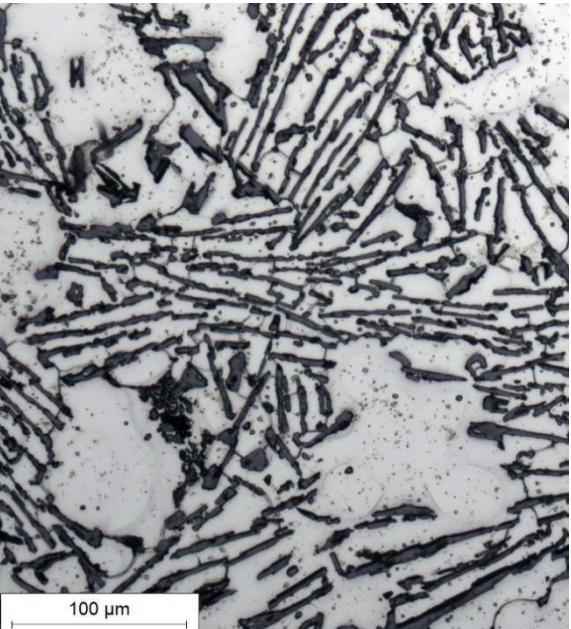
A micrograph showing a highly developed and dense network of dark, elongated precipitates, characteristic of a eutectic structure. A scale bar at the bottom left indicates 100 μm.<br>100 μm                                            |
