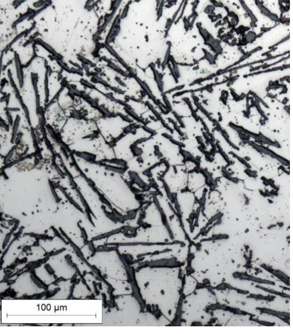
A micrograph showing a more randomly oriented and less aligned distribution of dark, elongated precipitates compared to the polished surface. A scale bar in the bottom left corner indicates 100 μm.<br>100 μm |
