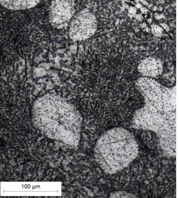
A micrograph showing a more complex and irregular distribution of precipitates compared to the polished surface, with some larger, darker regions and more scattered particles. A scale bar at the bottom left indicates 100 μm.<br>100 μm |
