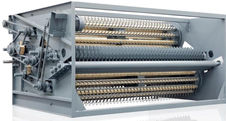
Slika 20. Bunch-Picking Machine SZ [42]
