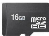
**Note:** A microSD card capable of SPI is a requirement for all 4D Systems’ display modules powered by Goldelox, Picasso or Diablo16 Processors. If a non-SPI compatible card is used, it will simply fail to mount, or may cause intermittent issues resulting in lock ups and crashing of the application. Please refer to the 4D Systems website for microSD cards offered by 4D Systems.
