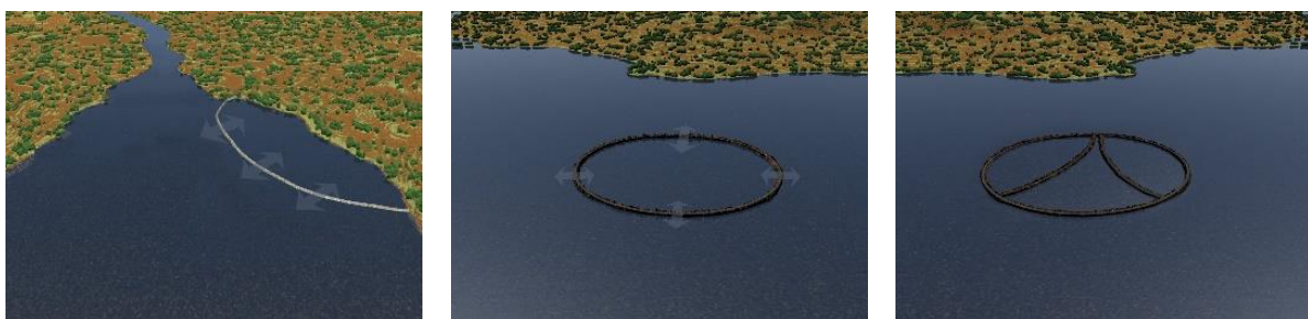
Figure 13. Tidal lagoon (left), single basin offshore tidal lagoon (middle) and multiple basin offshore tidal lagoon (right) [45]
