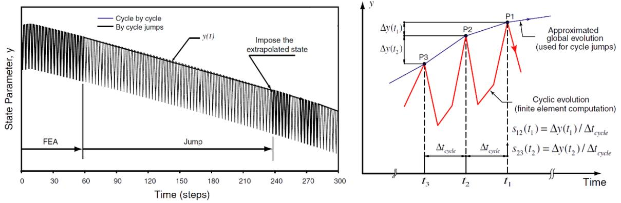
Fig. 3.3. Schematic representation cycle skipping technique [165]
