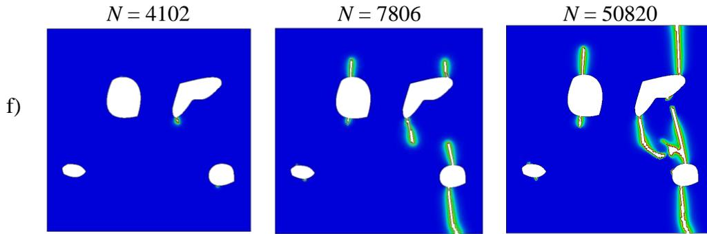
**Fig. 5.18. Cyclic loading. Evolution of fatigue fracture for displacement amplitudes a)  $u_1 = 0.001$ , b)  $u_2 = 0.00075$ , c)  $u_3 = 0.0005$ , d)  $u_4 = 0.00035$ , e)  $u_5 = 0.0002$ , and f)  $u_6 = 0.0001$**
