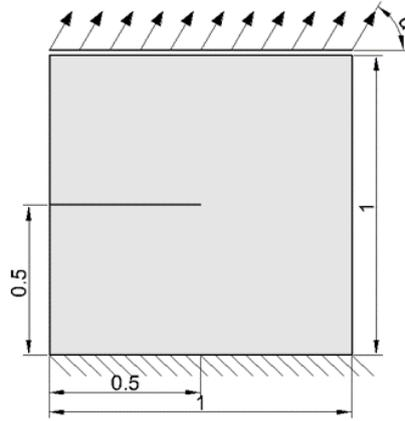
Fig. 4.5. Single edge notched specimen geometry and boundary conditions.
