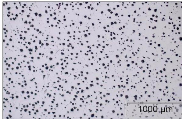
Fig. 5.1. Metallographic image of EN-GJS-400-18-LT microstructure [174]
