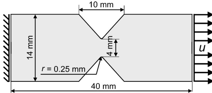
**Fig. 4.20. V-notch bar. Geometry and boundary conditions**
