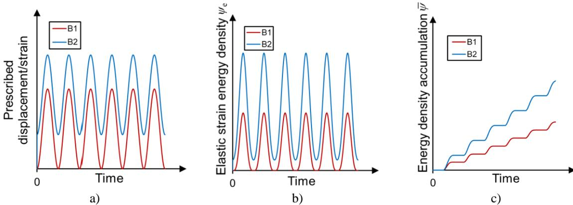
**Fig. 2.7. a) Prescribed load, b) resulting elastic strain energy and c) energy accumulation variable of 1D bar subjected to sinusoidal displacement-controlled loading with different mean values**
