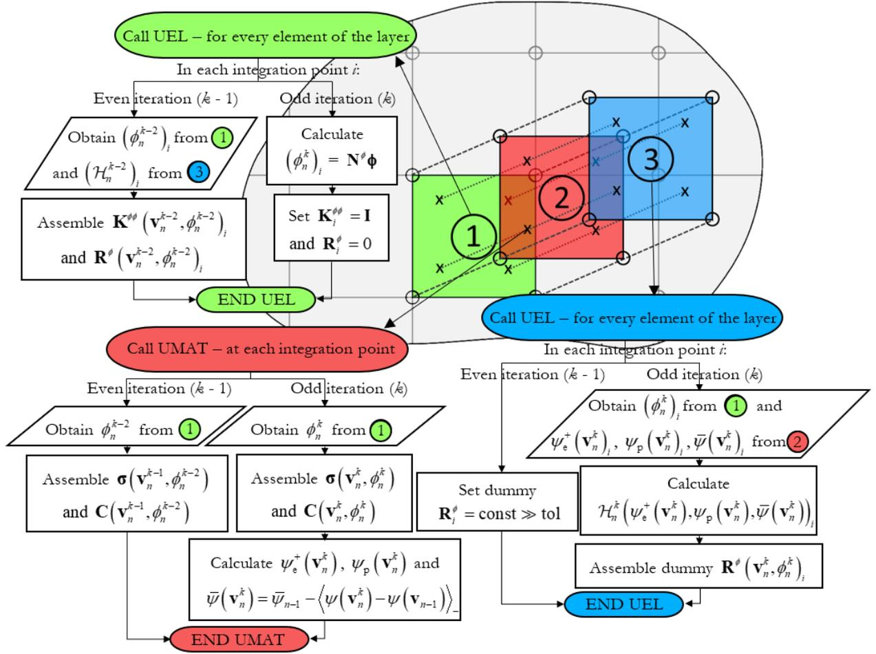
Fig. 3.2. ABAQUS implementation of the three-layered system
