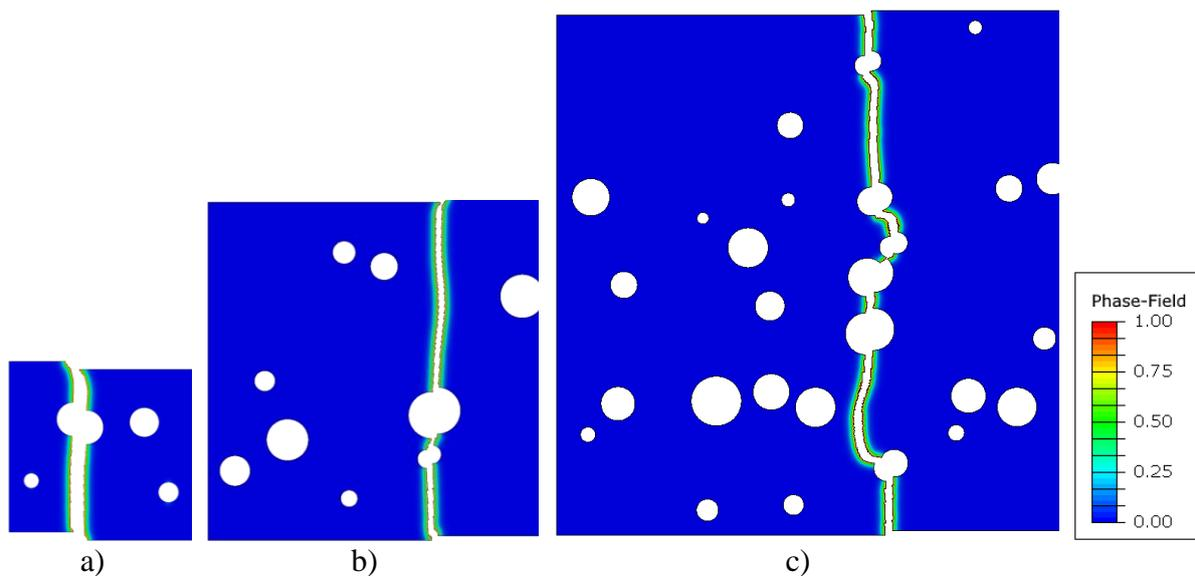
**Fig. 5.11. Monotonic loading. Brittle crack pattern obtained with N1 nodule modelling option on different specimen sizes (scale factor 20 is applied for better visualization)**
