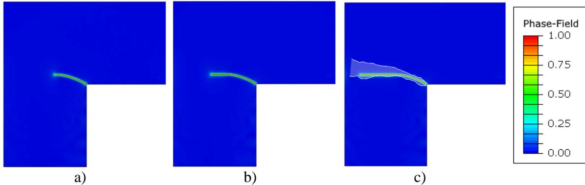
**Fig. 4.13.** L-shaped specimen. Crack pattern obtained by the spherical-deviatoric energy decomposition at a)  $u = 0.265$  mm, b)  $u = 0.3$  mm, c)  $u = 0.5$  mm with experimental envelope from [167]
