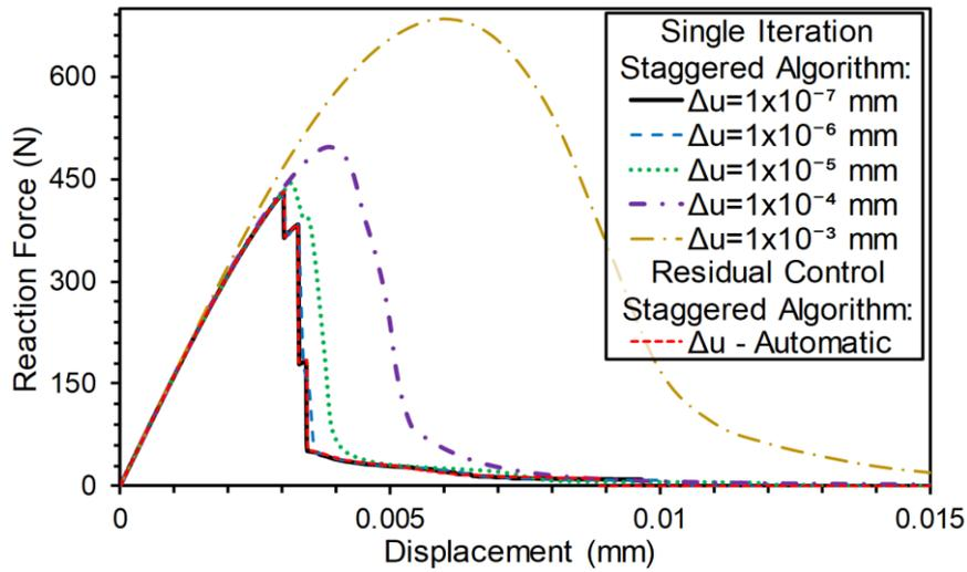
Fig. 4.18. Porous steel microstructural specimen. Force-displacement curves
