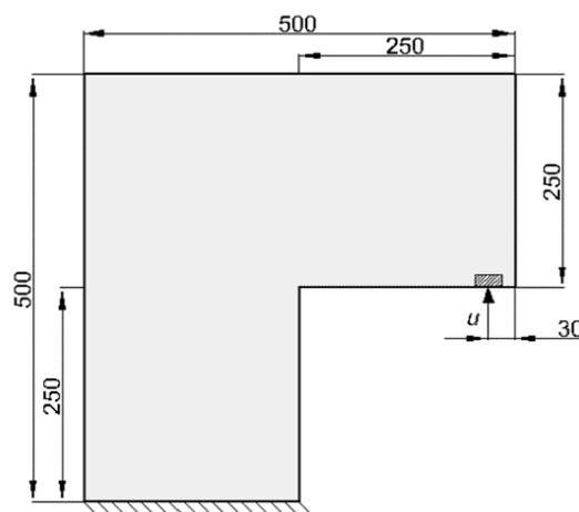
**Fig. 4.12. L-shaped specimen. Geometry and boundary conditions**
