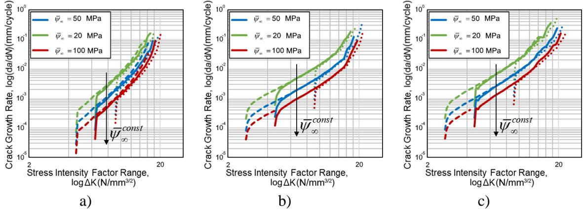
**Fig. 4.46.** Fatigue parameter  $\bar{\psi}_\infty$  influence on crack rate growth versus stress intensity factor change for fatigue degradation function a)  $\hat{F}_1$ , b)  $\hat{F}_2$ , and c)  $\hat{F}_3$
