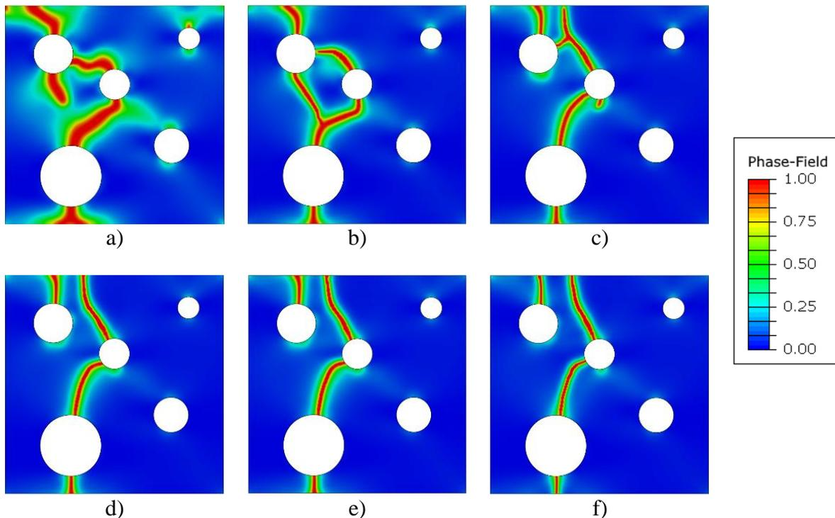
Fig. 4.19. Porous steel microstructural specimen. Crack patterns obtained by SI staggered algorithm with: a)  $\Delta u = 1 \times 10^{-3}$  mm, b)  $\Delta u = 1 \times 10^{-4}$  mm, c)  $\Delta u = 1 \times 10^{-5}$  mm, d)  $\Delta u = 1 \times 10^{-6}$  mm, e)  $\Delta u = 1 \times 10^{-7}$  mm, and f) RCTRL algorithm with automatic loading incrementation
