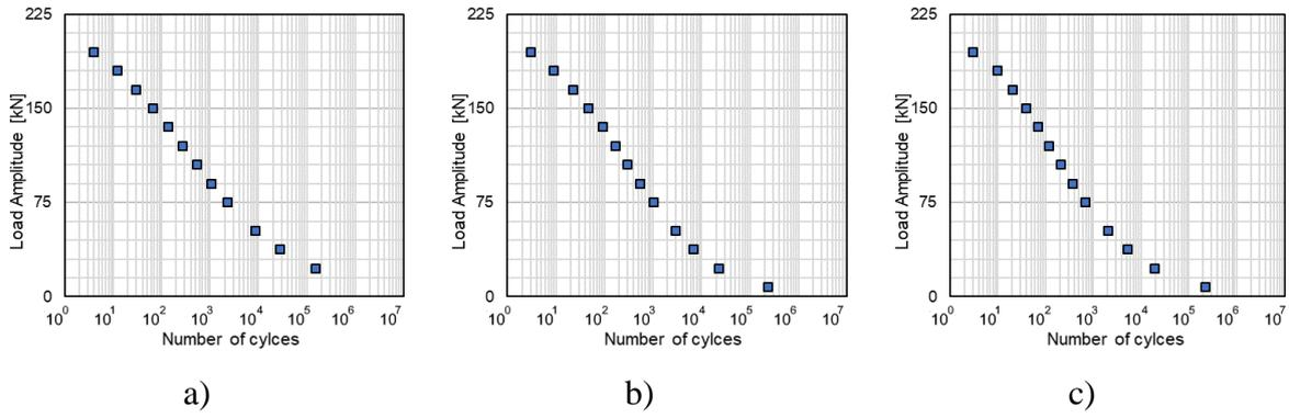
Fig. 4.42. Fatigue life for a)  $\hat{F}_1$ , b)  $\hat{F}_2$ , and c)  $\hat{F}_3$  fatigue degradation function
