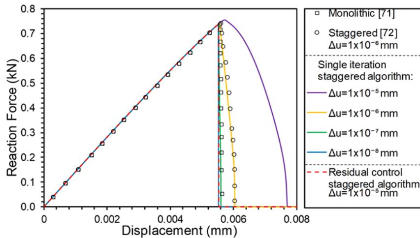
Fig. 4.7. Single-edge notched tension test. Force-displacement curves
