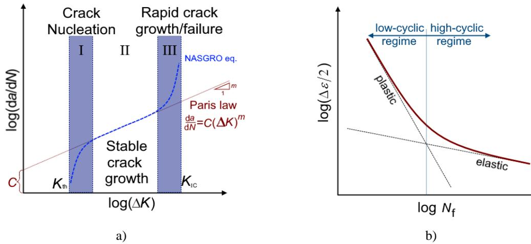
**Fig. 2.5 a) Crack growth curve approximated by Paris law where  $a$  is the crack length,  $N$  presents number of cycles,  $K$  is stress intensity factor, while  $C$  and  $m$  are material properties, b) Strain-life curve where  $\Delta \epsilon$  is the load amplitude and  $N_f$  is the number of cycles to failure**
