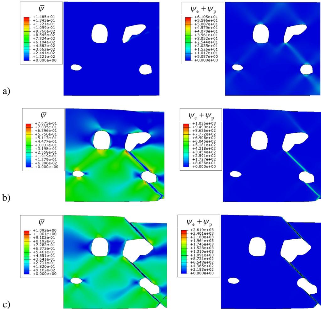
**Fig. 5.9. Monotonic loading. Total energy density and energy density accumulation variable plot at timeframes when a) no damage have yet started, b) the localization bands have formed c) final fracture frame occurs**
