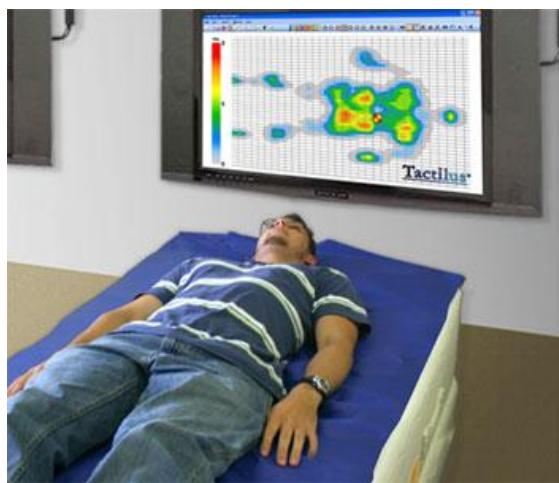
Slika 31. Tactilus® Bodyfitter® Full Body Sensor [19]
