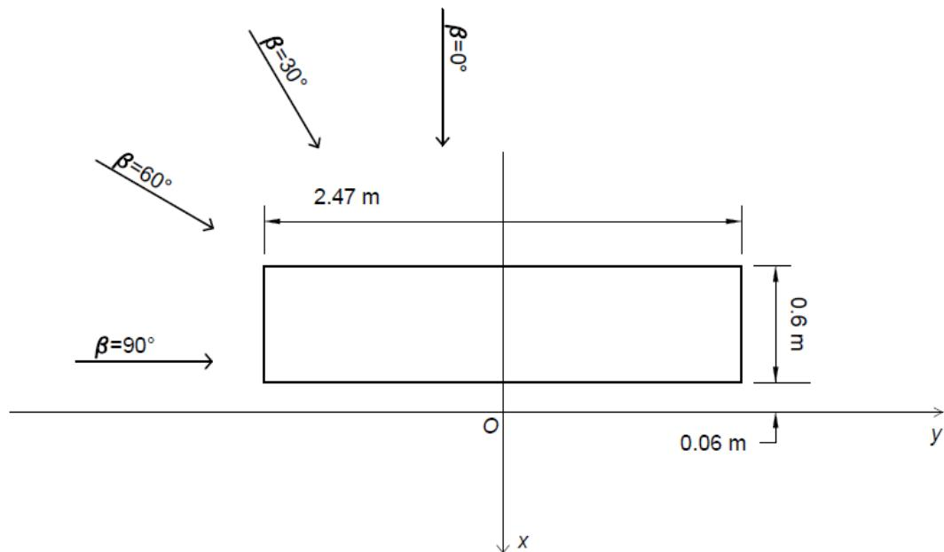
Slika 8. Dimenzije pontona *pntM06*
