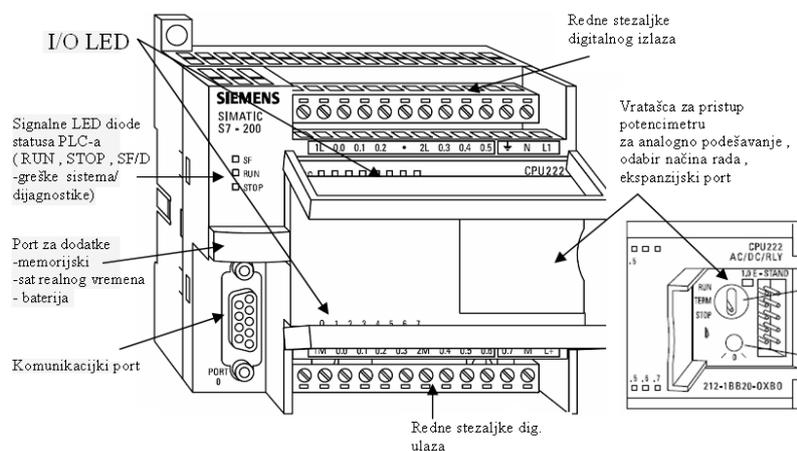
Slika 2.1 S7-200 PLC model CPU 224
