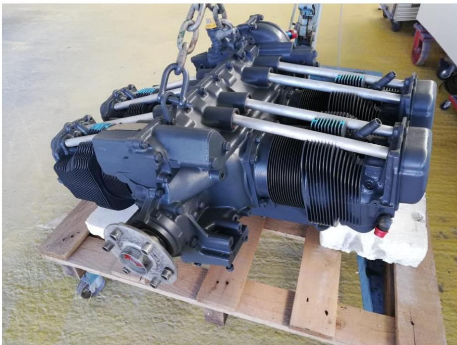
*Slika 2.3. Motor zrakoplova Cessna 172N Skyhawk Lycoming O-320-H2AD
