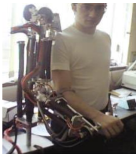
Slika 15. 7DOF Salford University „Soft actuated“ exoskeleton robot [20]
