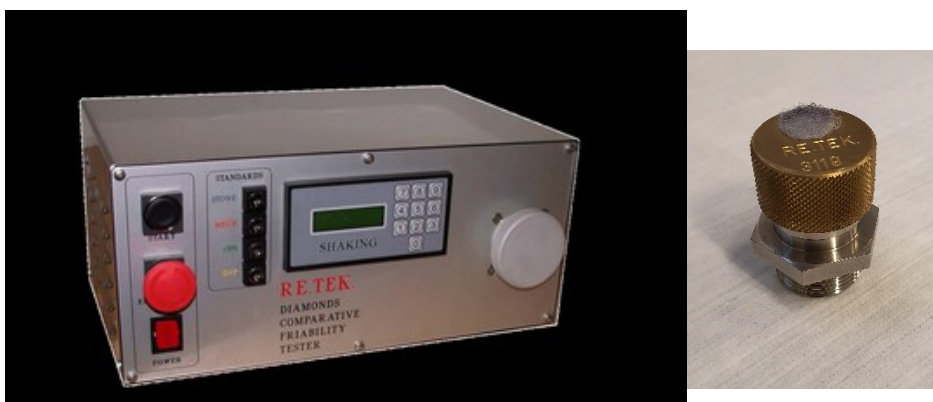
Figure 31: Friability tester from ReTek company with capsule [23]
