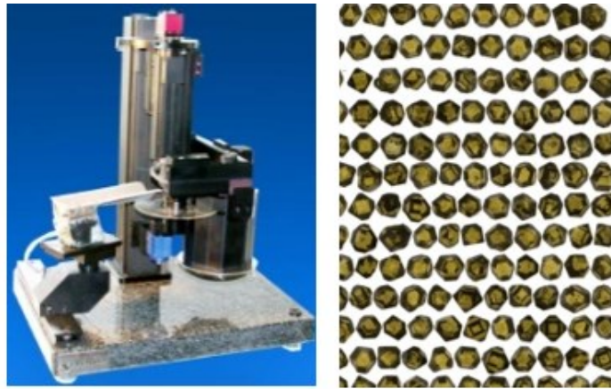
Figure 21: Optical image analysis with example of captured diamonds [21]
