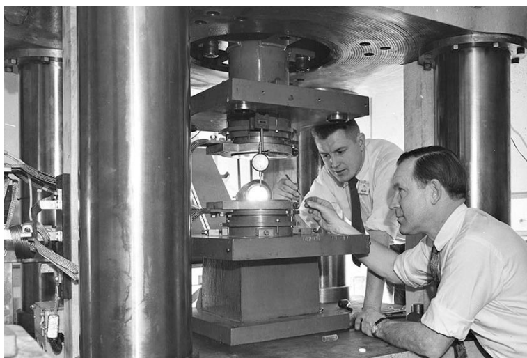
Figure 3: General electric builds a diamond making press in 1954. [5]
