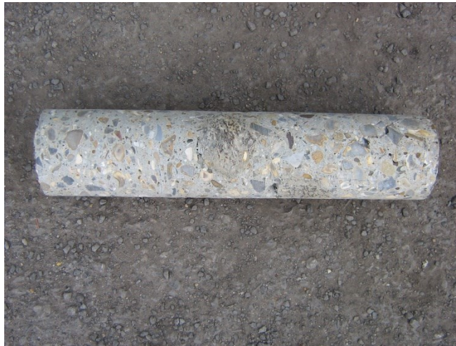
Figure 36: Concrete core sample taken for testing
