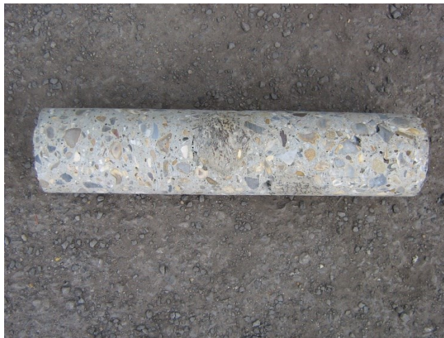
Figure 36: Concrete core sample taken for testing
