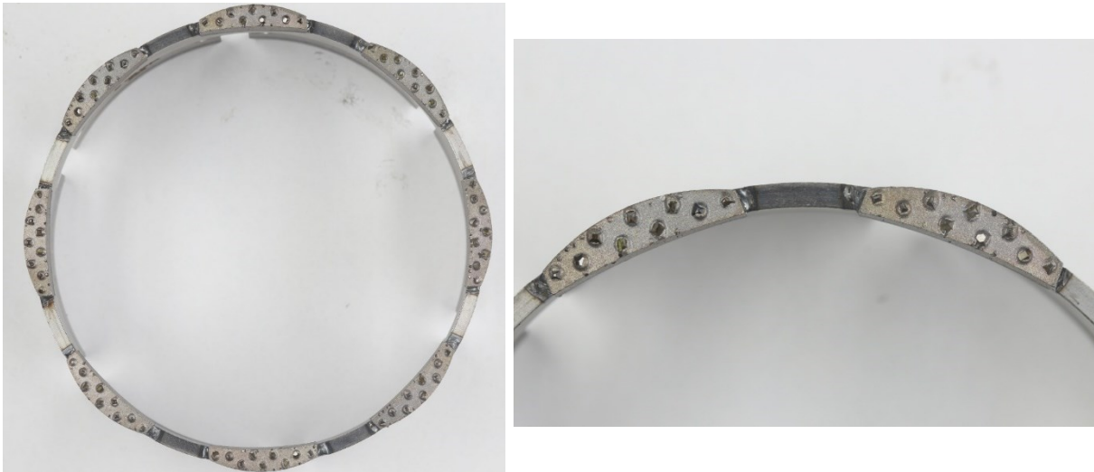
Figure 51: X-change module with visible large diamonds
