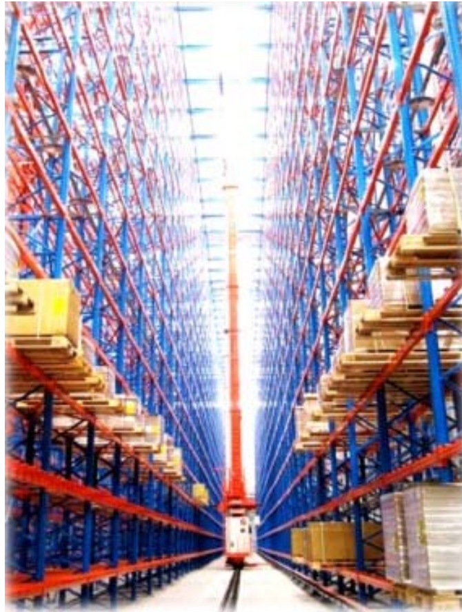
Slika 17. Unit-load S/R dizalica (Direct industry)
