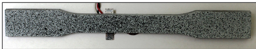
(a) Speckle pattern on the dog-bone sample
