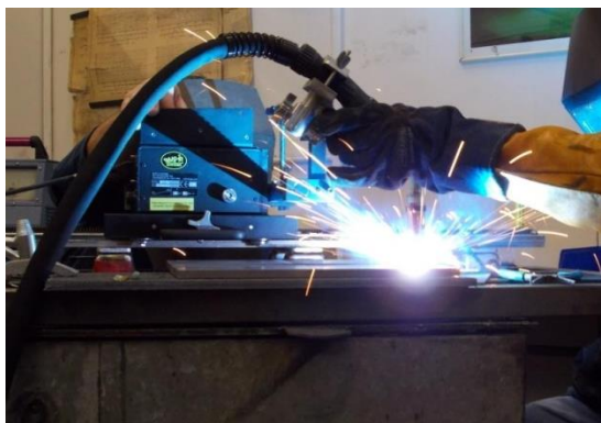
Slika 4.4 Automat BUG-O Systems MDS 1002
