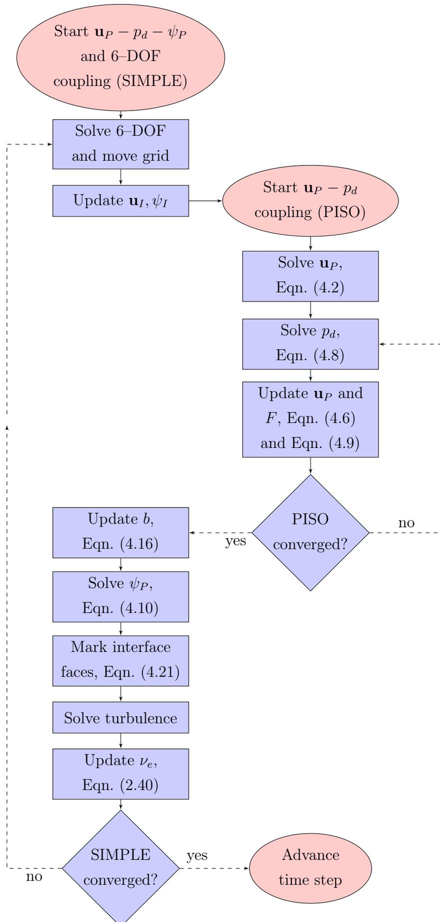
Figure 4.4: Flow chart of the segregated solution algorithm.
