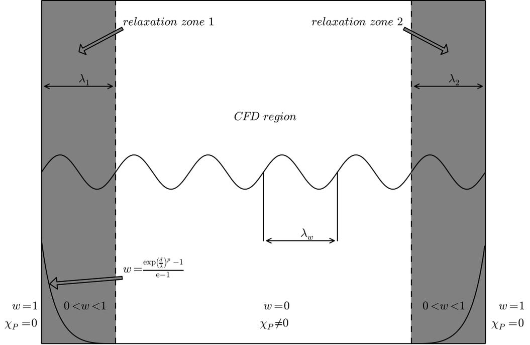
Figure 3.1: Relaxation zones with qualitative weight field function. The white region represents full CFD domain, while the shaded gray region represents relaxation zones. Within relaxation zones, the solution is a linear combination of calculated CFD solution and prescribed incident flow solution.
