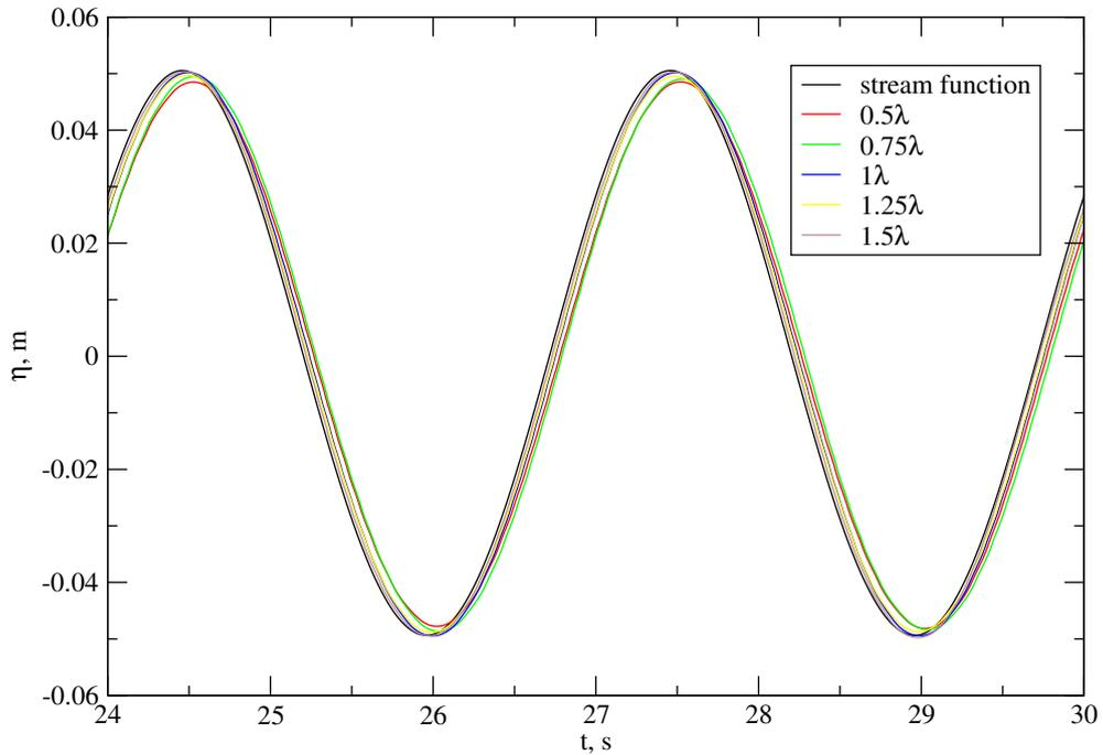
Figure 6.14: Time domain signals for last two periods, different relaxation zone lengths,  $\lambda_r$ .
