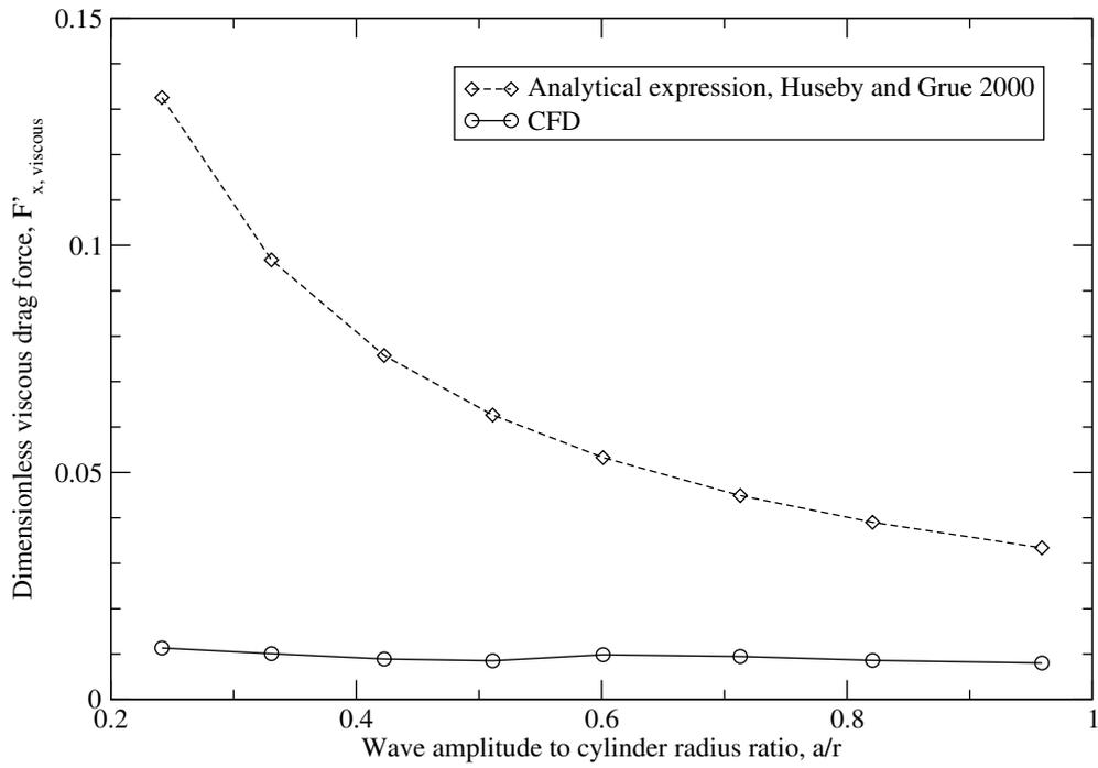
Figure 6.40: Comparison of dimensionless viscous drag forces.
