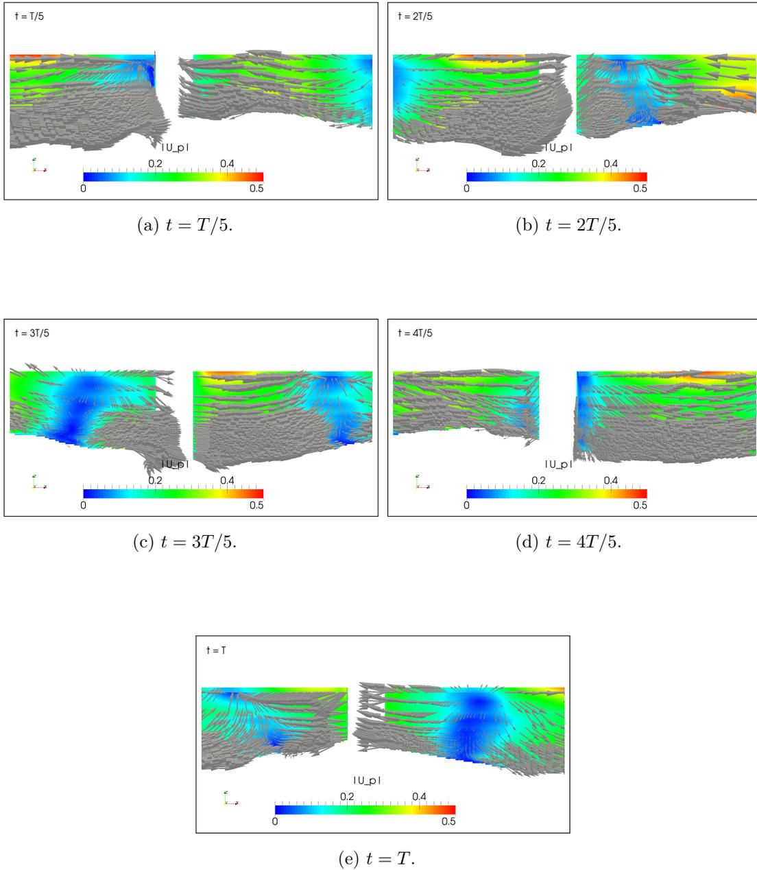
Figure 6.47: Perturbation velocity field ( $\mathbf{u}_P$ ) near the cylinder in air during the last (15<sup>th</sup> period),  $ka \approx 0.2$  case.
