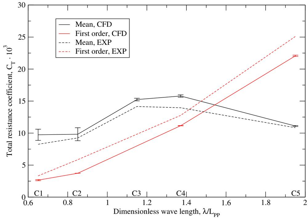
(a) Total resistance coefficient transfer function,
