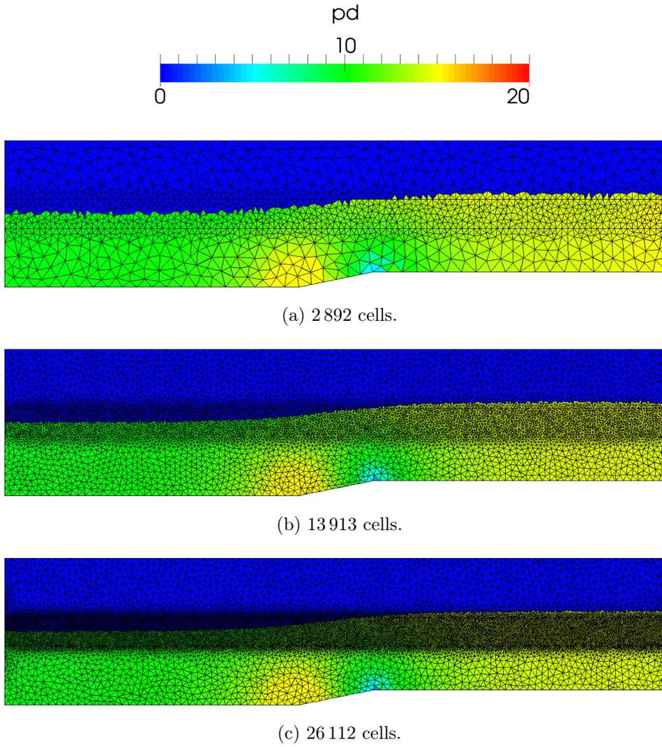
Figure 6.3: Dynamic pressure  $p_d$  at the steady state solution for three unstructured prismatic grids, approximately denoting the free surface due to presence of a sharp jump.
