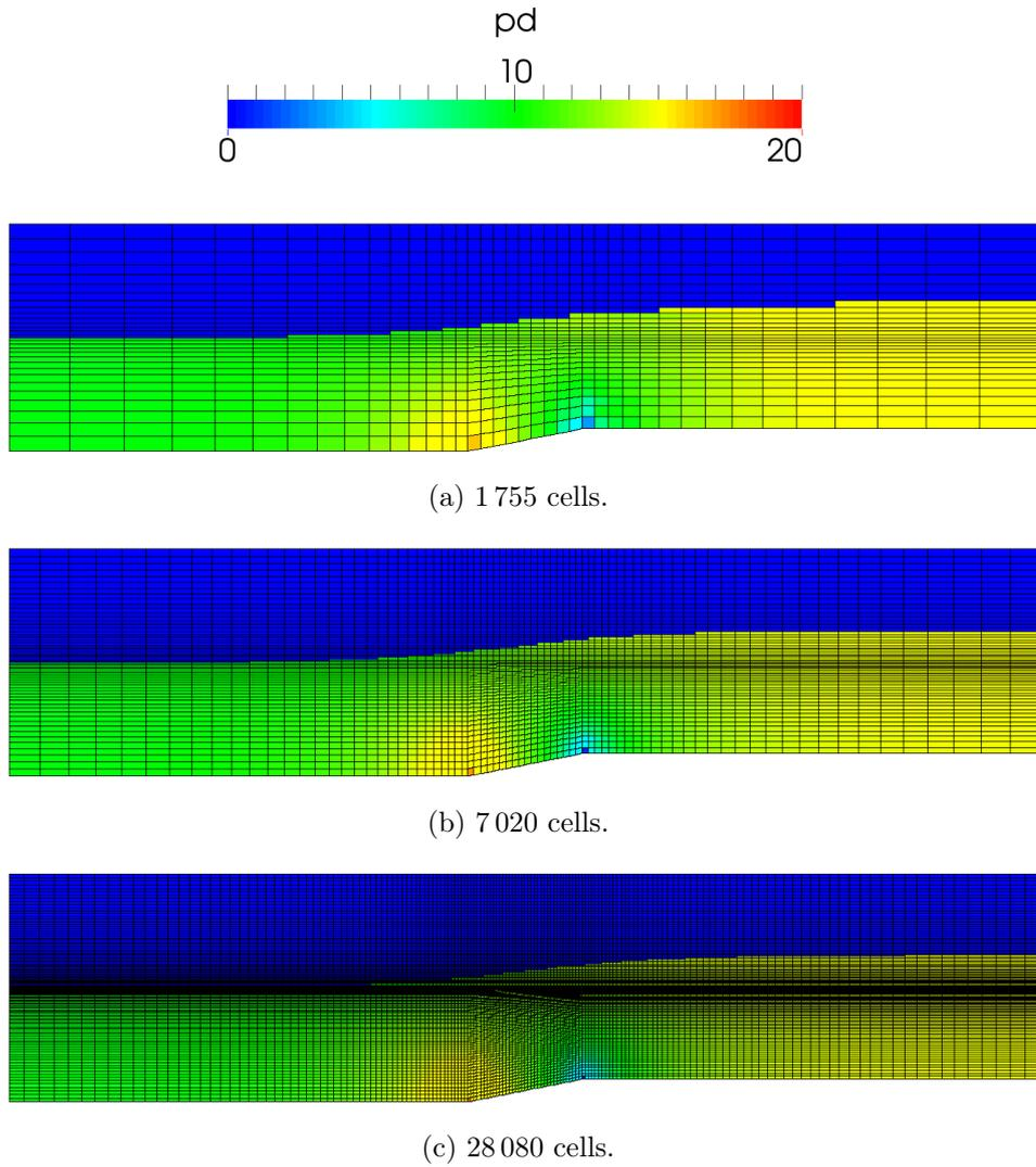
Figure 6.2: Dynamic pressure  $p_d$  at the steady state solution for three structured hexahedral grids, approximately denoting the free surface due to presence of a sharp jump.
