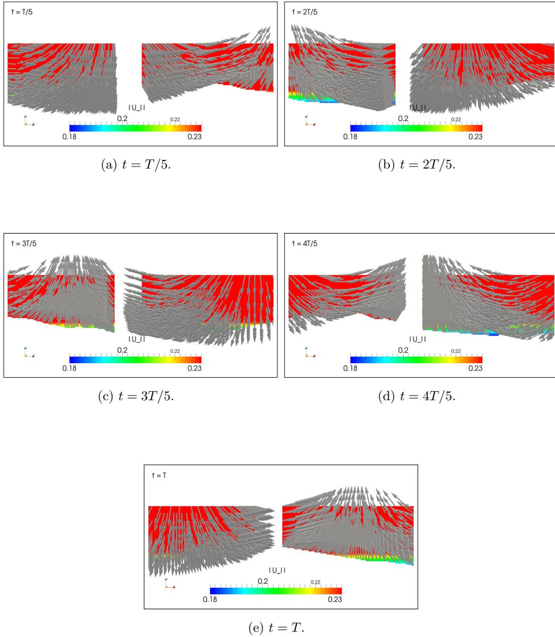
Figure 6.46: Incident velocity field  $(\mathbf{u}_I)$  near the cylinder in air during the last (15<sup>th</sup>) period),  $ka \approx 0.2$  case.
