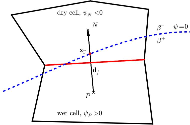
Figure 4.3: Compact polyhedral computational stencil near the free surface. Free surface is denoted with the blue dashed line. Interface face shared by cells  $P$  and  $N$  is marked with a red line, and the location of the free surface is denoted with  $\mathbf{x}_\Gamma$ .
