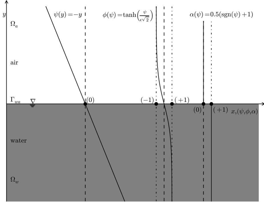
Figure 2.1: Comparison of interface capturing schemes.  $\psi$  is the signed distance function for the LS field,  $\phi$  is the PF and  $\alpha$  is the volume fraction in the VOF approach.
