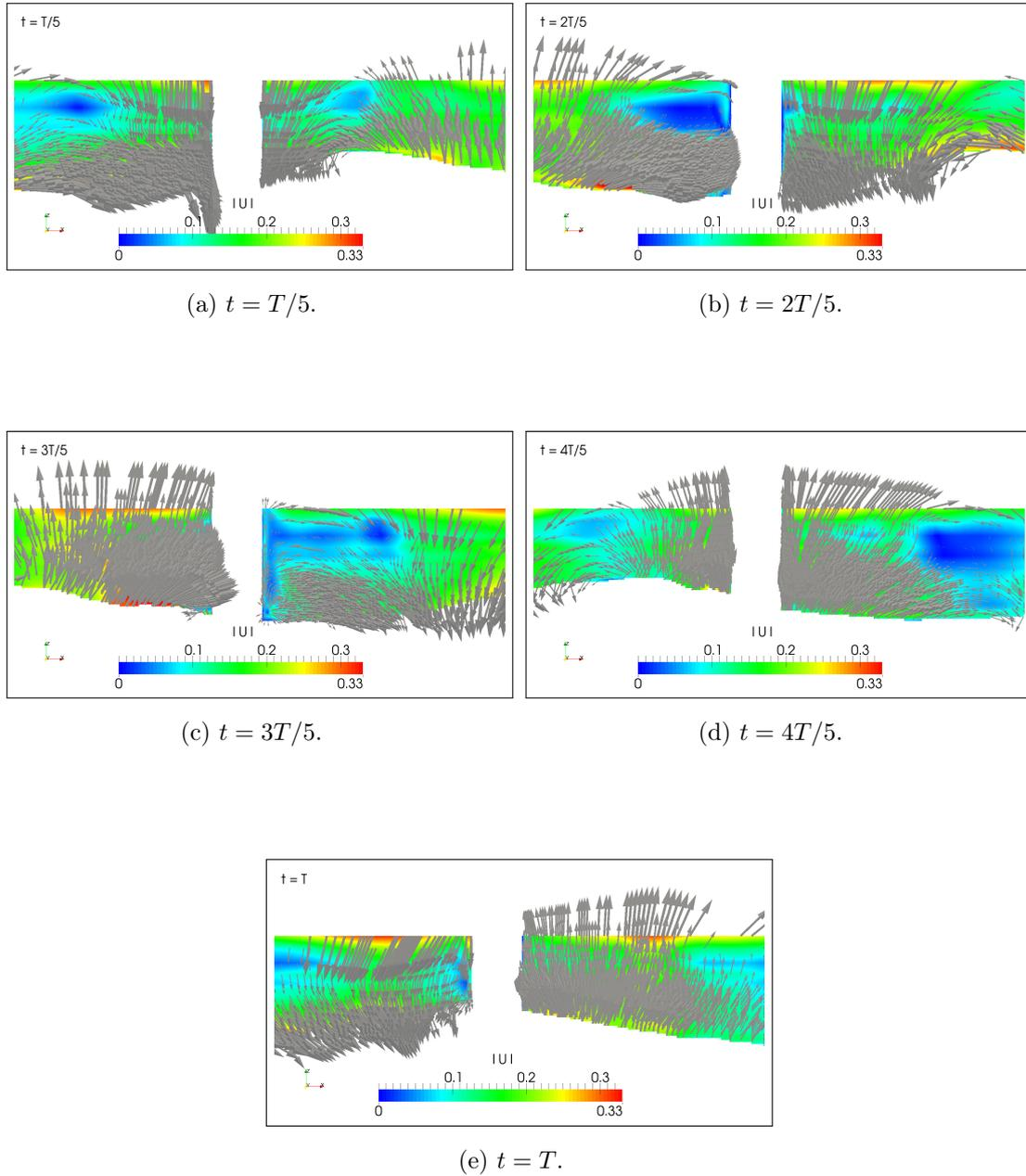
Figure 6.48: Total velocity field ( $\mathbf{u} = \mathbf{u}_I + \mathbf{u}_P$ ) near the cylinder in air during the last (15<sup>th</sup> period),  $ka \approx 0.2$  case.
