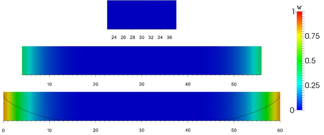
Figure 6.7: Weight field for wave propagation test case. The top image presents the area where fully nonlinear, two-phase and viscous CFD solution is obtained. The middle image presents the area where there is 50 to 100% of the CFD solution. The bottom image presents the whole domain, where the black line in the bottom image is a qualitative representation of weight function Eqn. (3.14).
