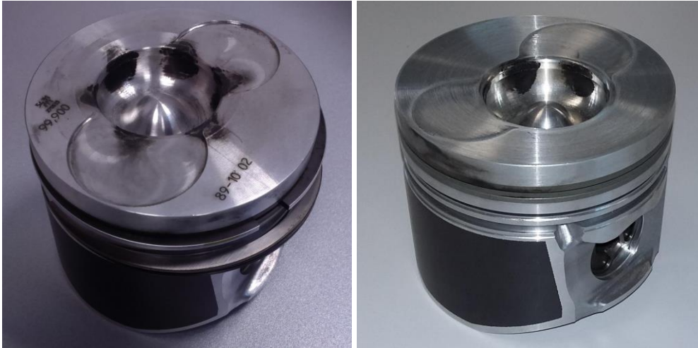
Figure 20. Left: original piston; right: after machining (-0.7 mm)
