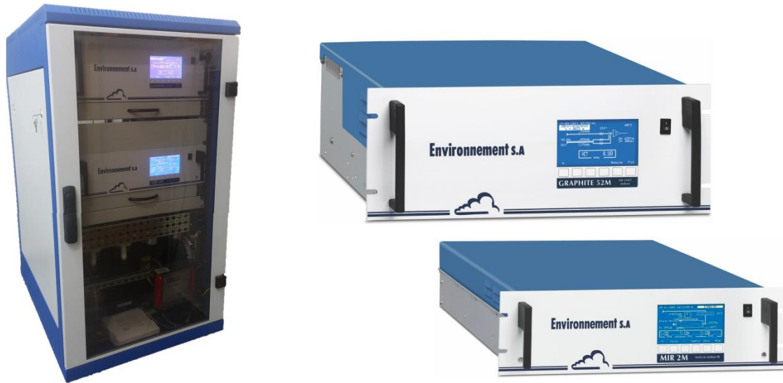
Figure 45. Analysers for THC; CO and CO 2 emission; reproduced from [83]
