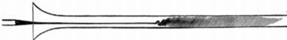
Figure 1.2: The Reynolds experiment, the tube filled with a mass of coloured water [1]
