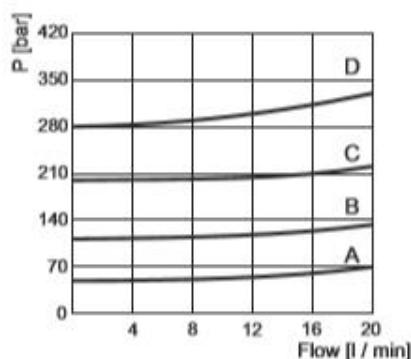
Note: Values measured on valve alone (no cavity) with an oil viscosity of 46 cSt at 50 °C. Pressure drop may change depending on fluid viscosity and temperature
