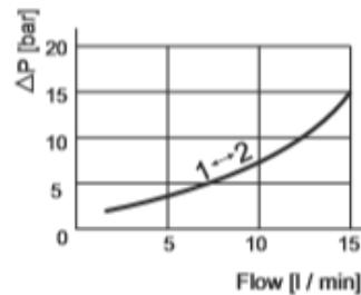
Note: Values measured on valve alone (no cavity) with an oil viscosity of 46 cSt at 50 °C. Pressure drop may change depending on fluid viscosity and temperature
