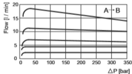
Note: Values measured on valve alone (no cavity) with an oil viscosity of 46 cSt at 50 °C. Pressure drop may change depending on fluid viscosity and temperature
