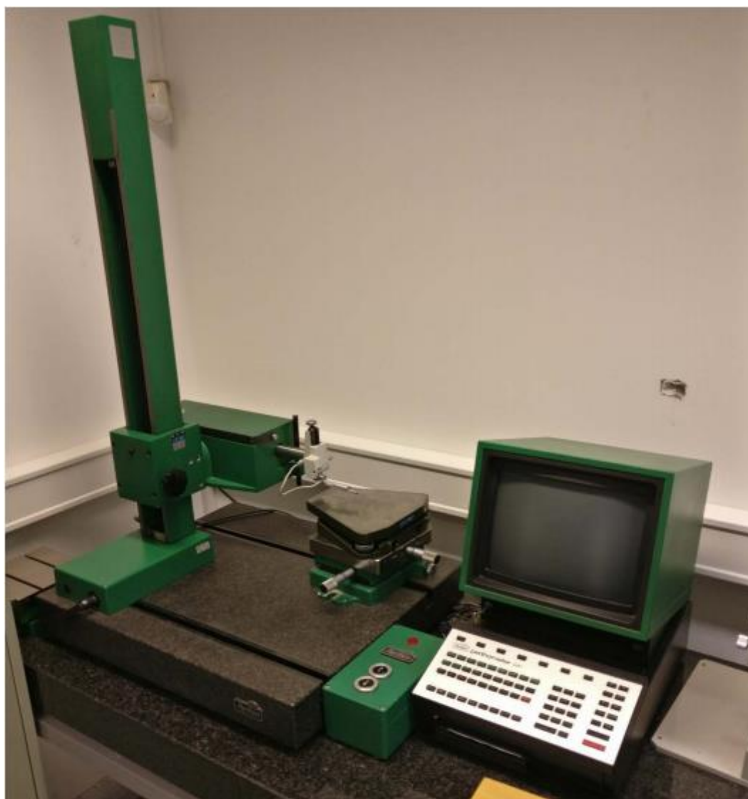
Slika 23. Mahr Perthen Perthometer S8P instrument s ticalom
