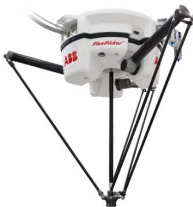
Slika 3. Delta robot ABB IRB 360 FlexPicker
