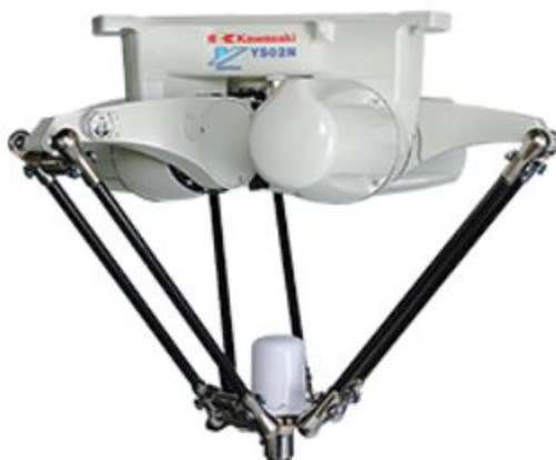
Slika 6. Delta robot Kawasaki Robot YF002N
