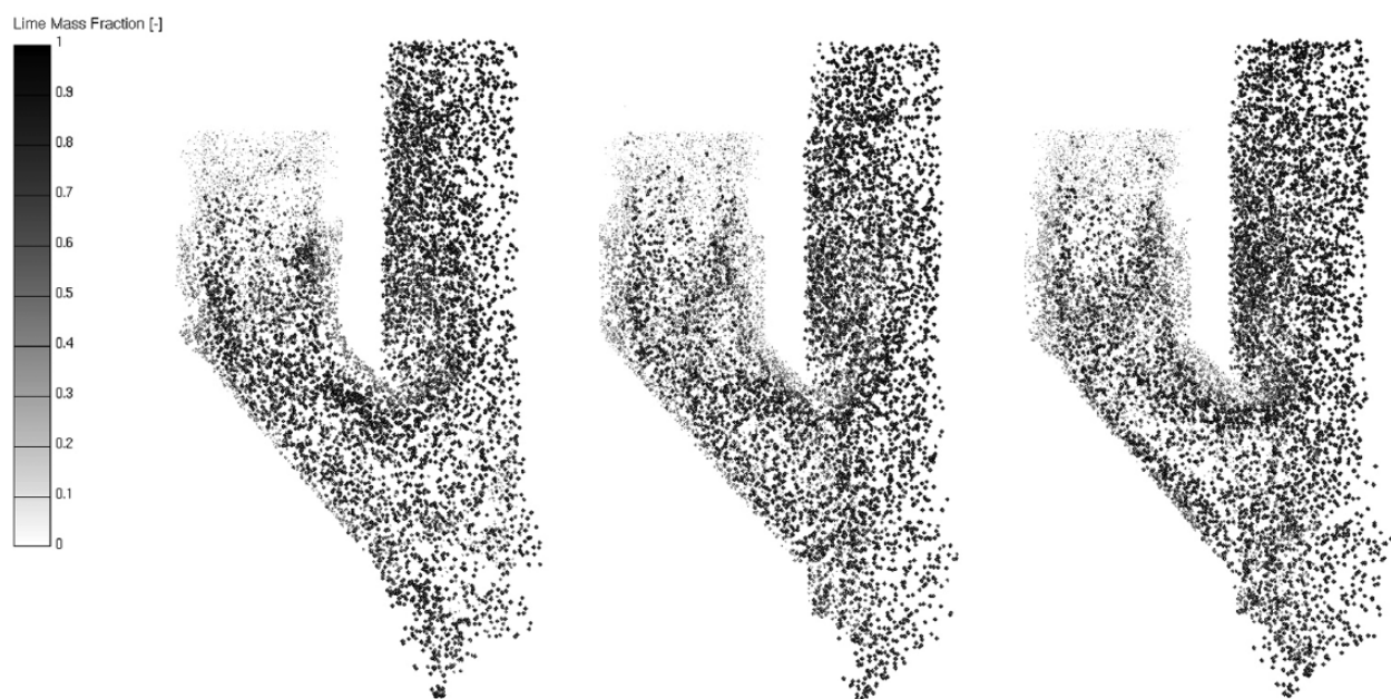
Figure 5. Lime ( \text{CaO} ) mass fraction in particles: Case 1 (left); Case 2 (middle); Case 3 (right).
