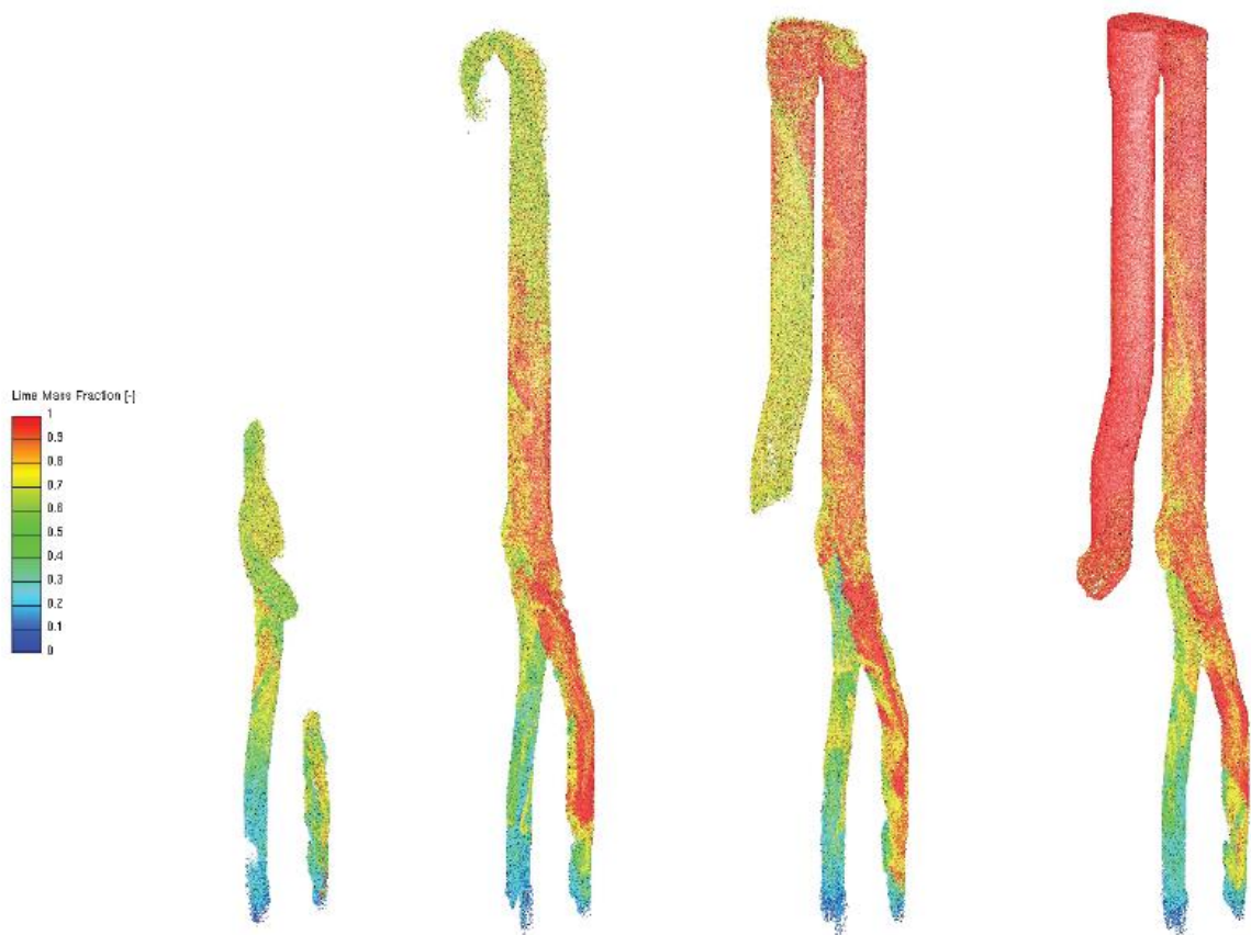
Figure 23 Lime production at different particle residence time: 2 s (left); 4 s (second from left); 6 s (second from right); 8 s (right).
