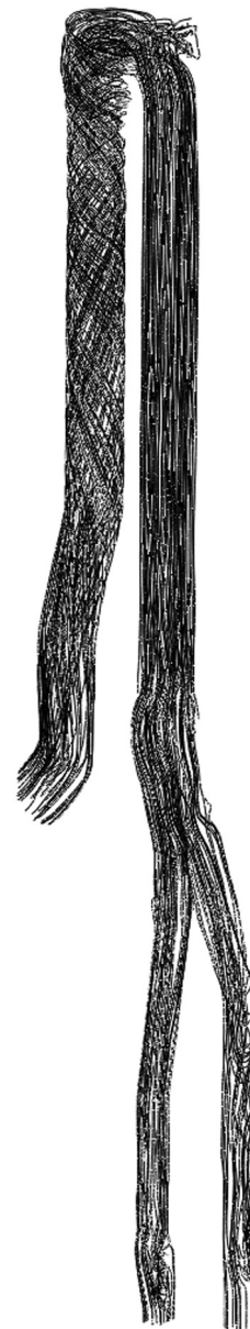
Fig. 2. Flow streamlines inside the calculated calciner.
