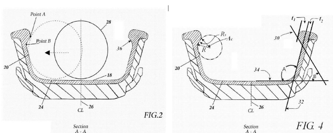
Slika 26 Patent US 8096613 B2 (eng. *Head restraining foam liner for car seat*) – prikaz 2 [37]
