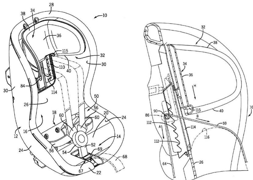
Slika 29 Patent CN 102341268 B (eng. *Child safety seat with height adjustable harness and headrest*) – prikaz 1 [37]
