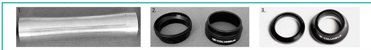
SLIKA 6 – 6.1 Head tube, 6.2 – kapice, 6.3 - ležajevi
