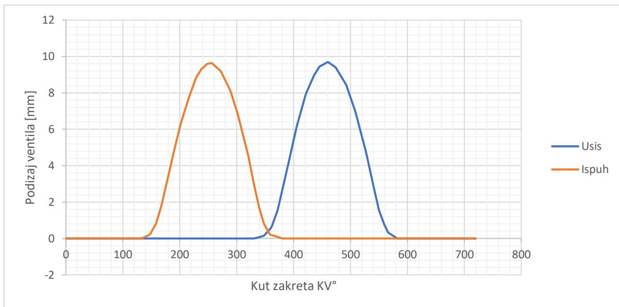
**Slika 8. Podizaj ventila**
