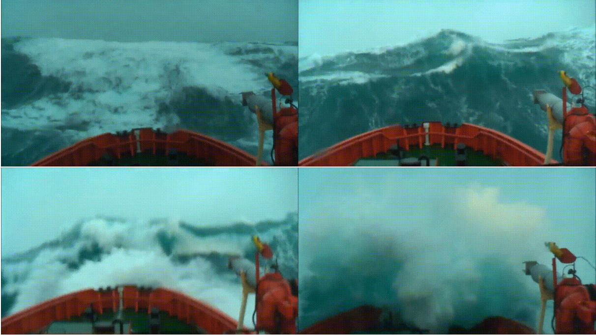
Figure 1.1.: A typical timeline of green water over the bow. The vessels heads into high waves that break just above the bow generating large amount of momentum.
