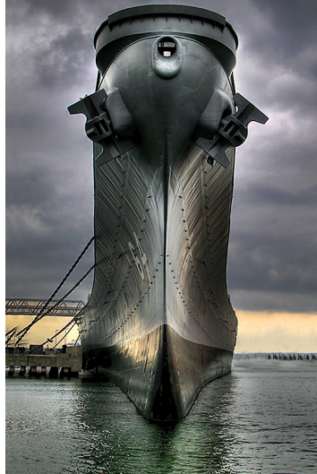
Figure 1.5.: Bow flare of USS Wisconsin at her berth in Norfolk, VA. Photograph taken by Steve Hersey.
