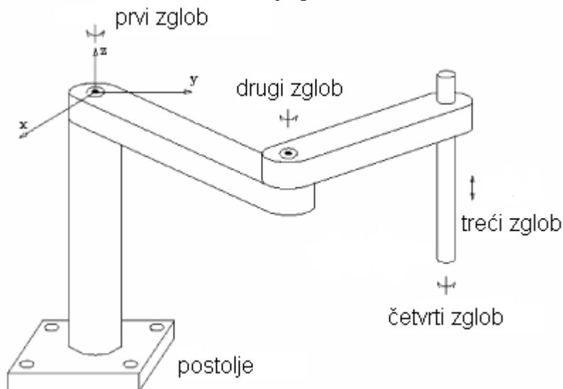
**SCARA - Selective Compliance Assembly Robot Arm.**
