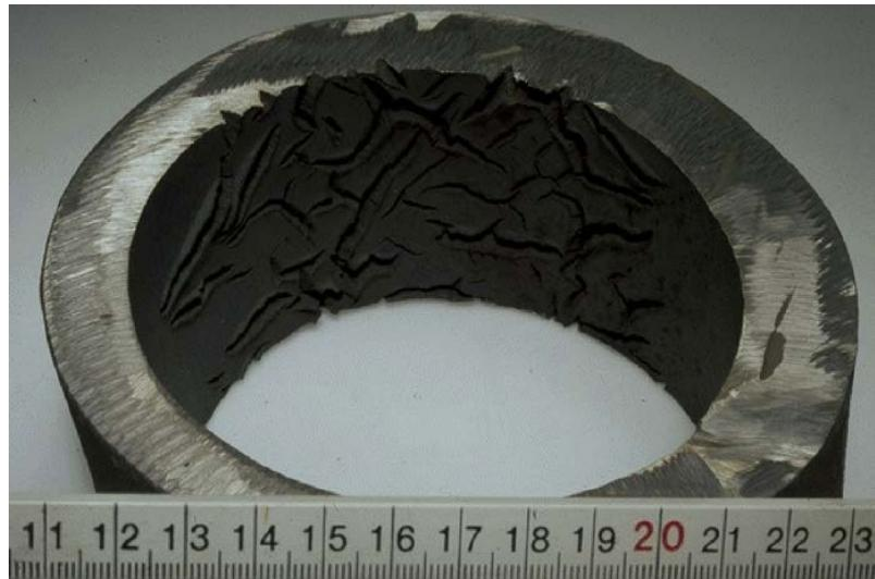
**Slika 9. Prikaz karburiranja legure ASTM H P40 [19]**
