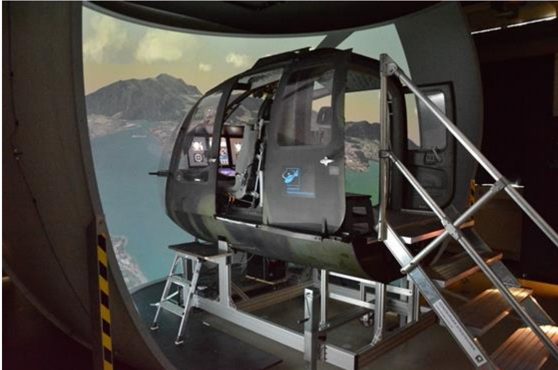
Figure 4 Exterior view on a flight simulator connected to ROSIE at Technical University of Munich [6]
