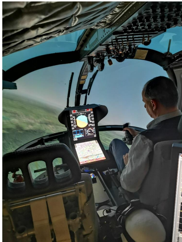
Figure 36 Simulator experiment with a pilot-in-the-loop in a Mission Task Element: Commanded roll PFD
