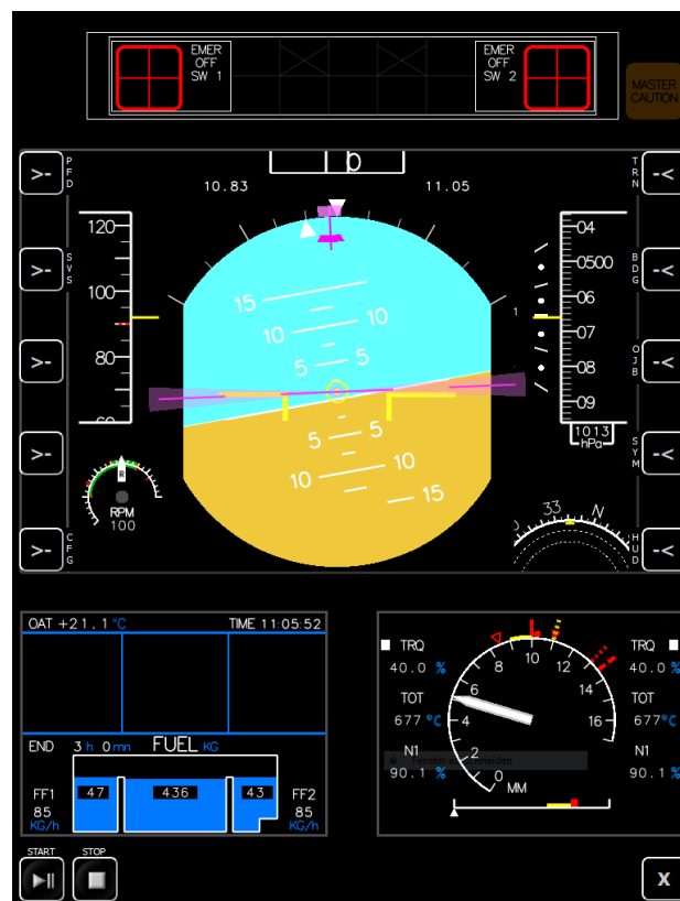
Figure 28 Primary flight display used for the experiment
