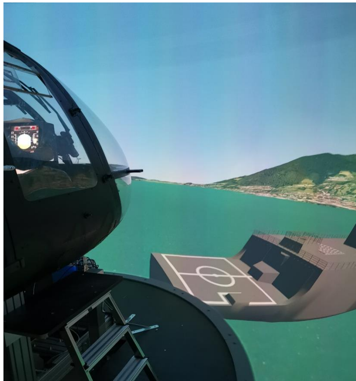
Figure 25 ROSIE visualization of DDG-51 type ship, rotorcraft landing deck
