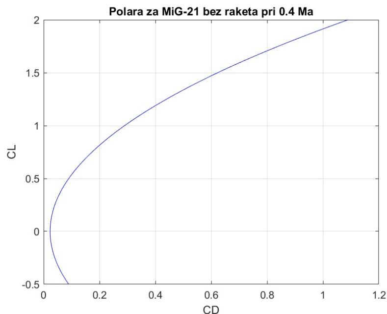
**Slika 5. Polara MiG-21 bez raketa**
