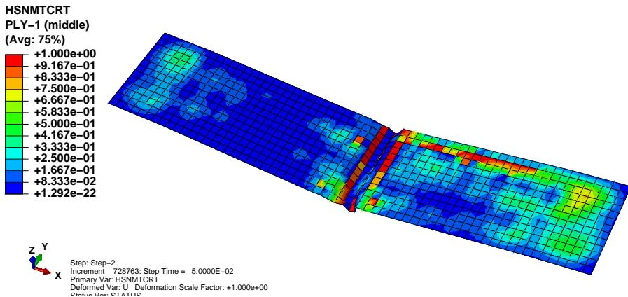
Slika 4.19: HSNMTCRT kriterij popuštanja za sloj  $0^\circ$
