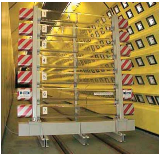
Fig. 2: Prototype of the barrier in the wind channel
