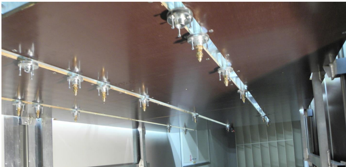
Figure 3.2 Climatic section with water sprinklers
