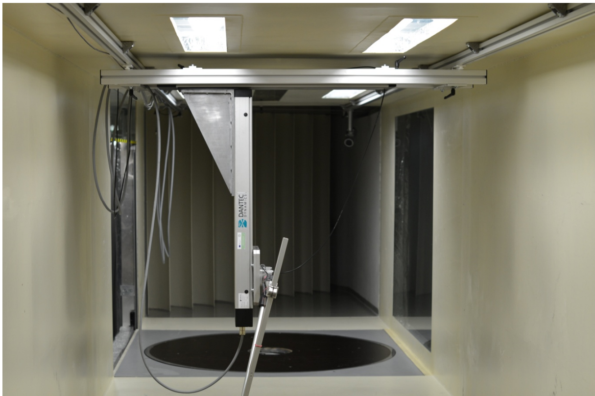
Figure 3.9 Dantec Dynamics traverse system in the aerodynamic test section
