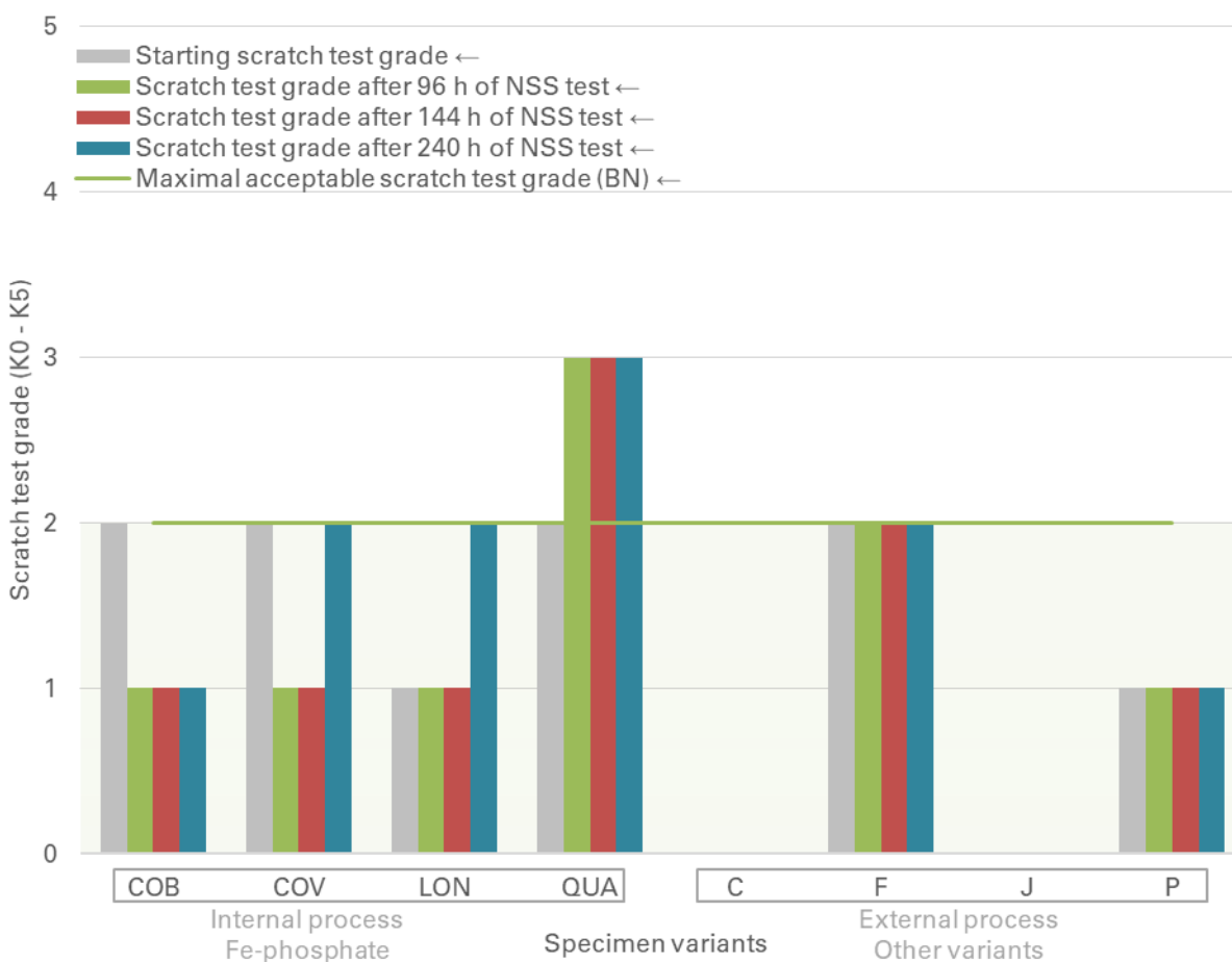
Figure 68. Comparison of scratch test results (colored bars) on CED coated specimens, after 96, 144 and 240 hours of the NSS test, in relation to initial values (grey bars) and different pre-treatment variants
