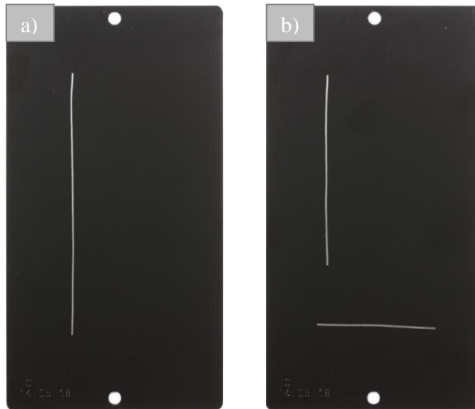
Figure 24. Sample scribe lines on a) steel and hot-dip galvanized steel specimens and b) aluminium specimens
