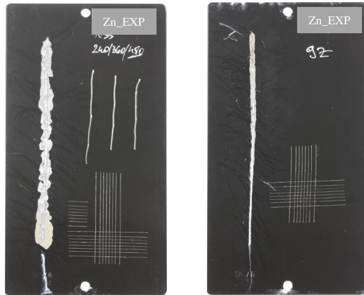
Figure 60. Zn_EXP specimens with adequate coating adhesion after 480 hours of NSS and 9 cycles of VDA-new test
