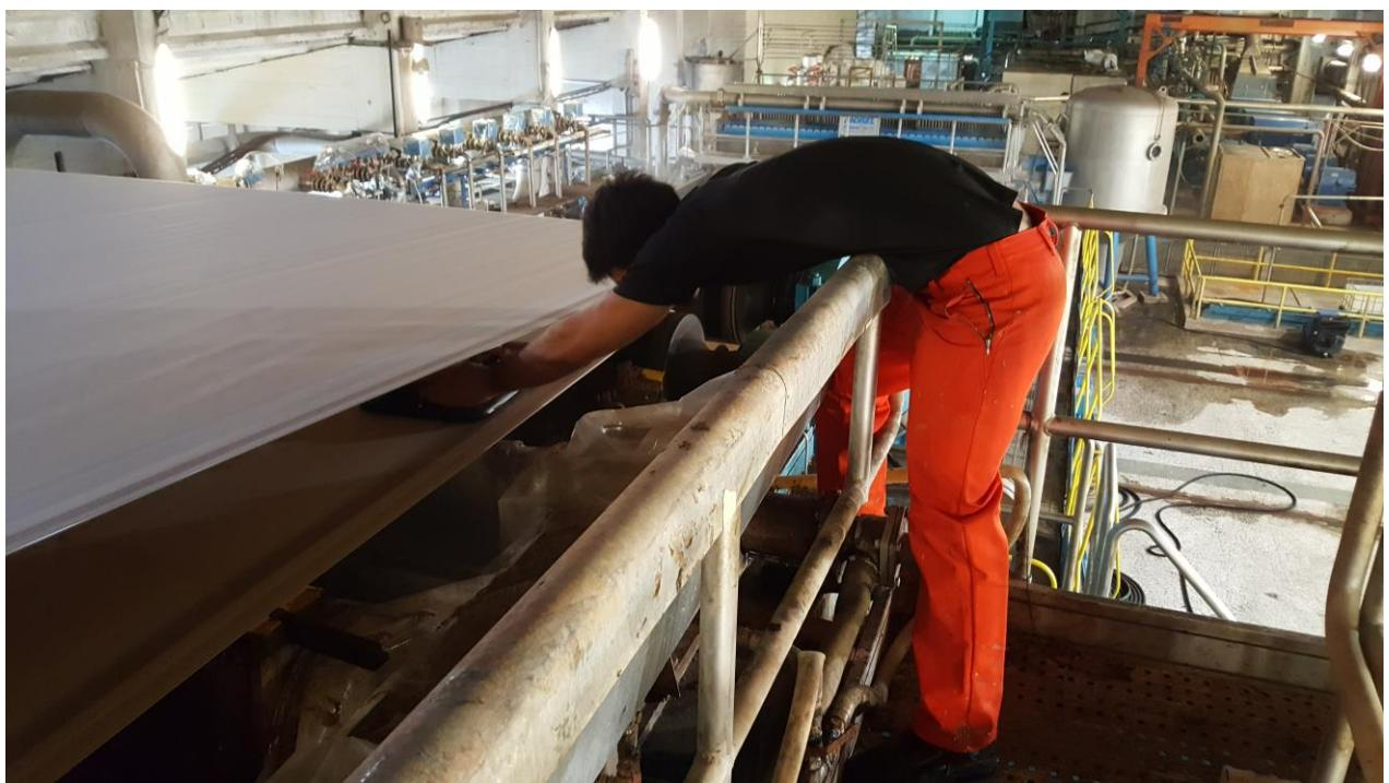
Slika 41. Machine direction after nip - Pick-up filc
