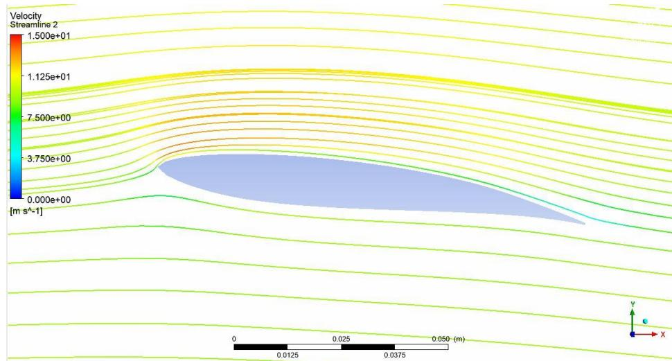
Slika 34. Strujnice  $\alpha = 8^\circ$ ,  $v_s = 10 \text{ m/s}$ , ravnina  $z = 0,5w$
