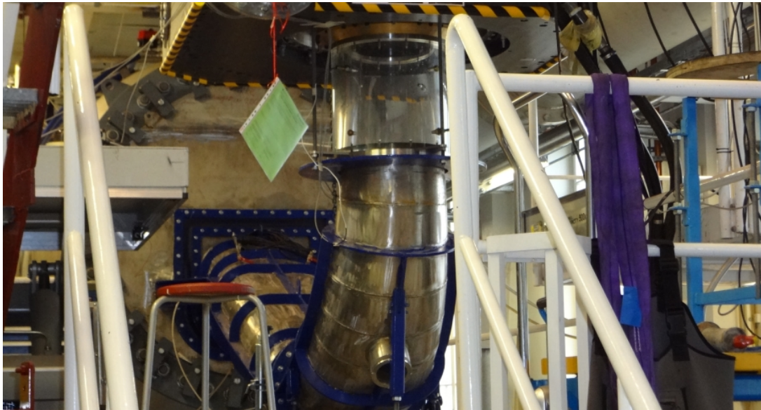
Figure 5.3.1: Test rig of the model Francis turbine/pump-turbine [19]
