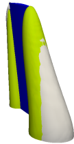
Figure 5.2.17: Onera M6 pressure = 15 Pa contour with an angle of attack of 5 degrees, yellow contour - IBM result, white contour - BF result
