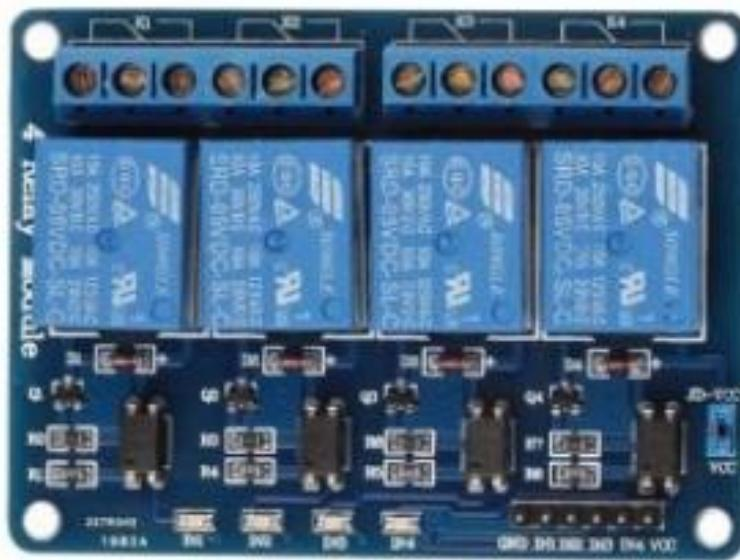
Slika 31. Relejni blok Songle SRD-05VDC-SL-C
