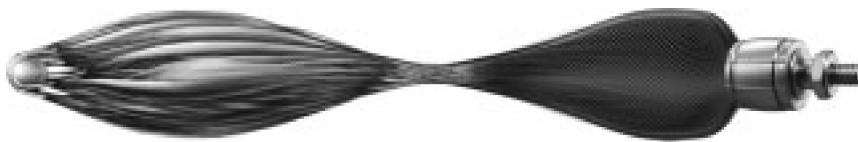
Fluidic Muscle is a tensile actuator which mimics the natural movement of a muscle. It consists of contractible tubing and appropriate connectors. The contractible tubing is made up of a rubber diaphragm with a non-crimped fibre made of aramid yarns on the inside. The diaphragm provides a hermetic seal enclosing the operating medium. The yarns serve as a reinforcement and trans-
