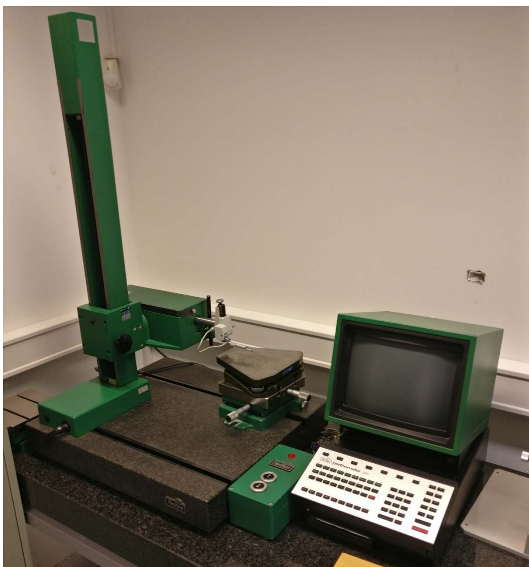
Slika 27. Mahr Perthen Perthometer S8P instrument s ticalom
