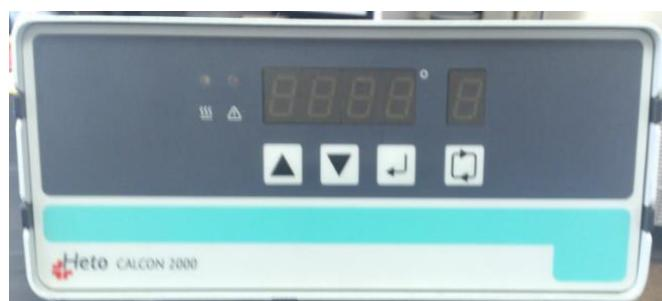
Slika 2. Calcon 2000 regulator temperature
