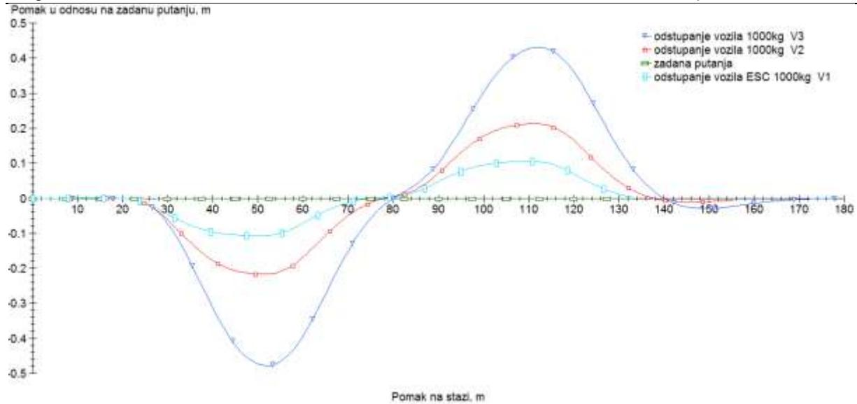
Slika 62. Bočni pomak vozila od zadane putanje bez brzine V<sub>4</sub>, CarSim
