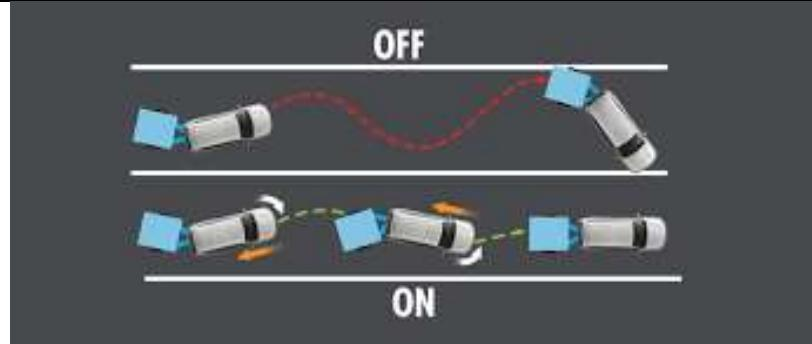
Slika 23 . Trailer stability assist način rada [25]
