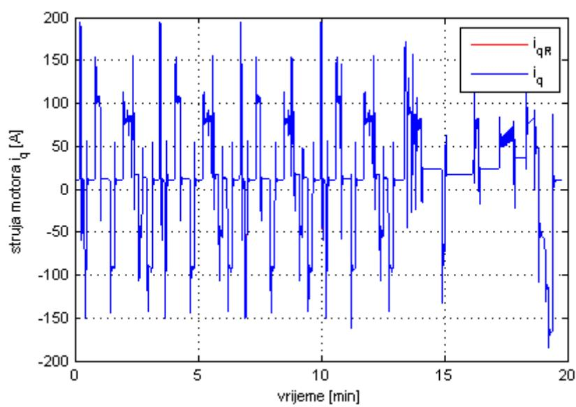
Slika 5-4 Struja  $i_q$  servomotora
