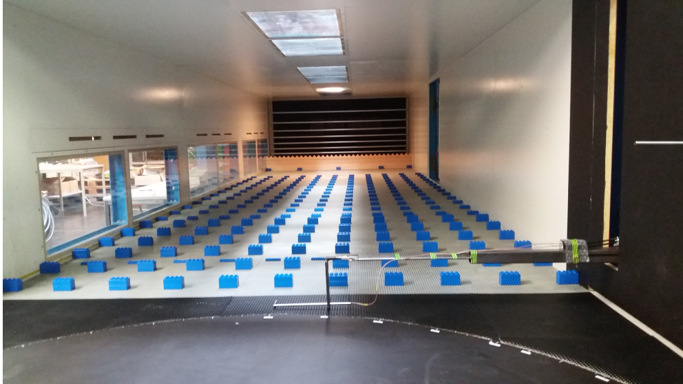
Figure 3.16: Hot-wire probe mounted on a traverse in the IFMHT-GUT wind tunnel
