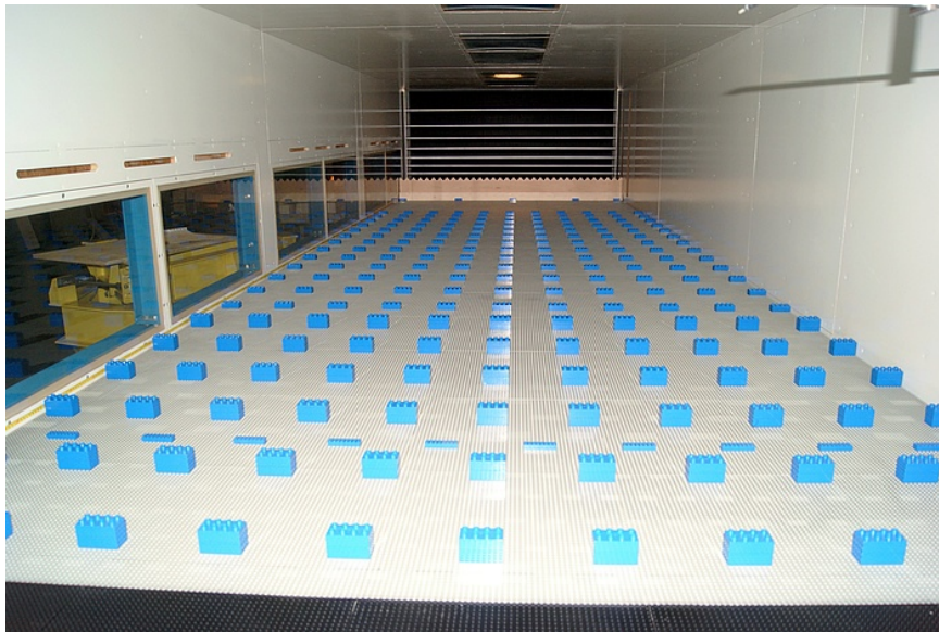
Figure 3.3: Test section floor covered with surface roughness elements, [23]
