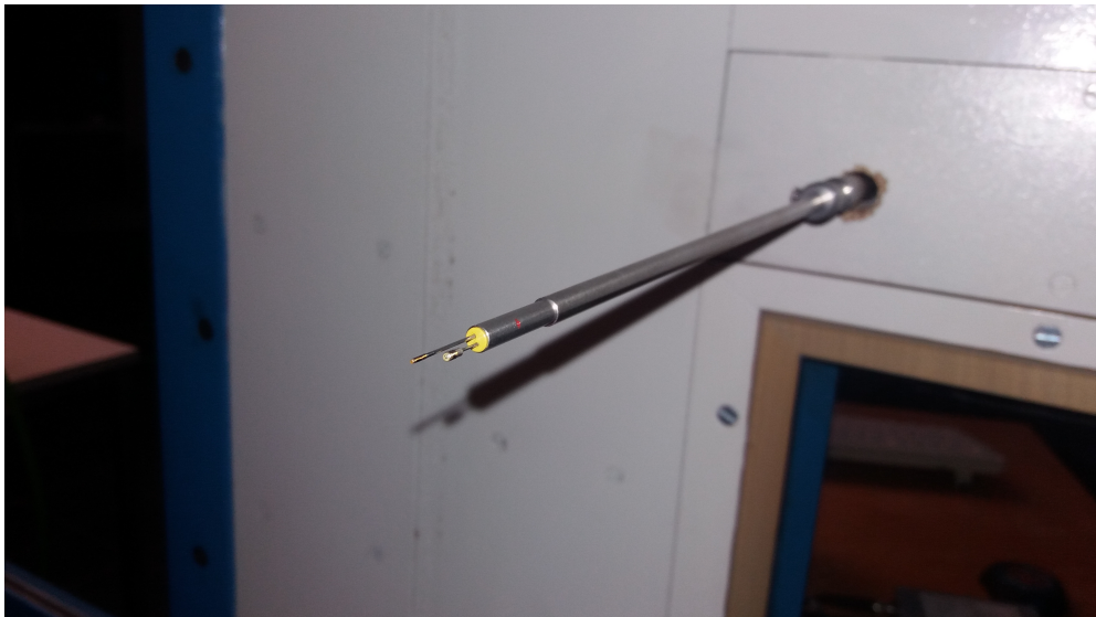
Figure 3.17: Reference velocity sensor 54T29 mounted on the IFMHT-GUT wind tunnel wall
