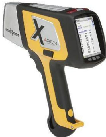
**Slika 29: Uređaj Delta Environmental Handheld XRF**
