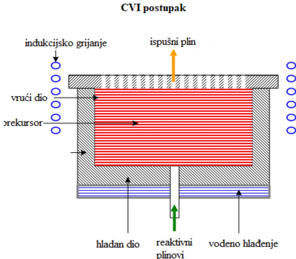
Slika 4.4 Postupak CVI (Chemical Vapour Infiltration) [15]
