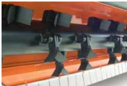
**Slika 45** Čekići na rotoru [10]
